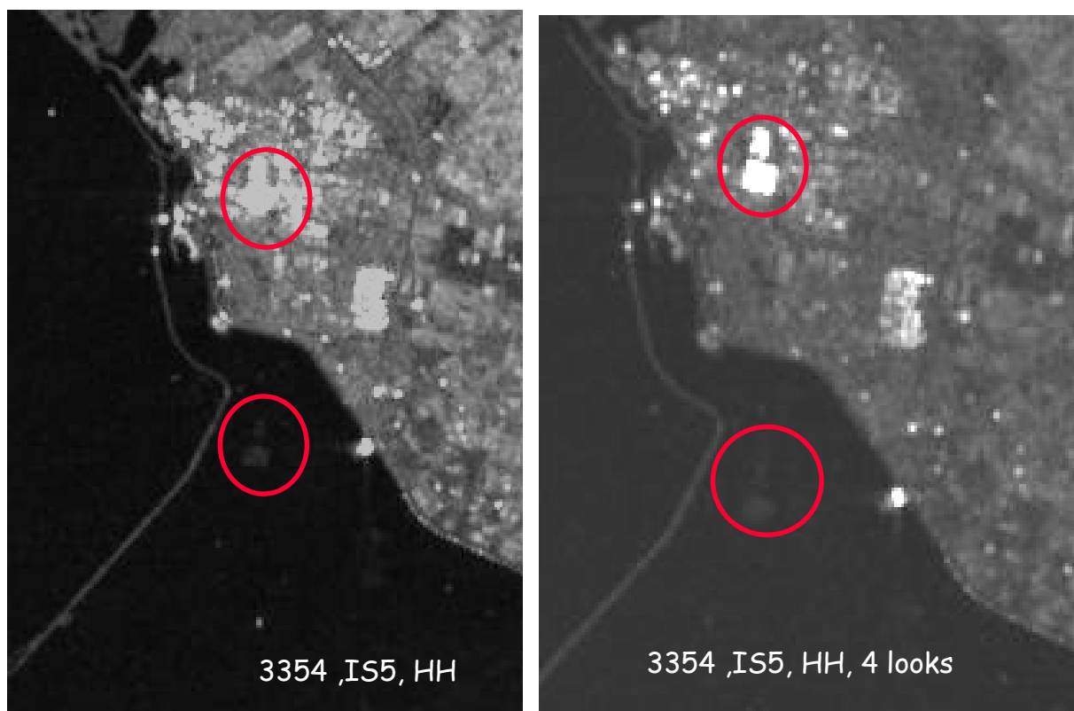
Fig. 9. IMM HH azimuth ambiguities (Left) Standard IMM processing with 10 azimuth looks. (Right) Special IMM processing with 4 azimuth looks.
