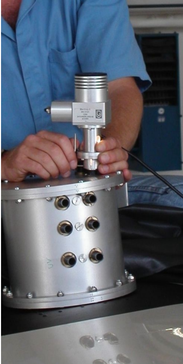
Fig. 2: Radiometric calibration of the AMAXDOAS optical telescopes
