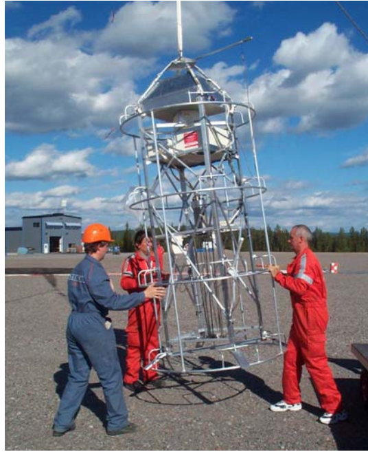
Fig.1. A picture of the SDLA balloonborne diode laser spectrometer during its flight from Kiruna on 8 August 2002 in the framework of the ENVISAT validation campaign.
