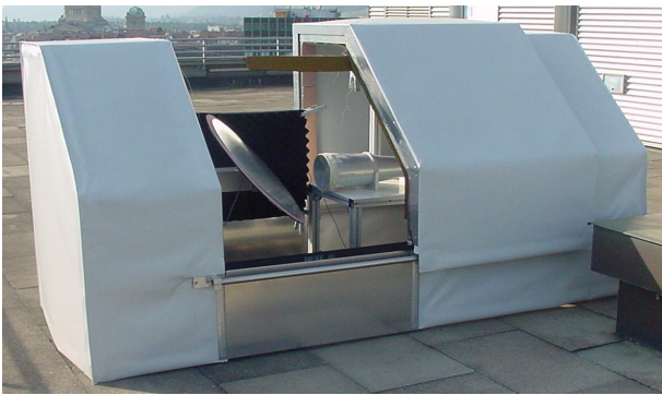
Figure 3. The microwave radiometer MIAWARA measures water vapor from 20 to 80 km altitude.
